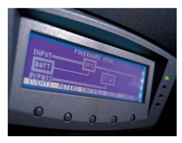
battery management systems to take the guesswork out of battery maintenance. Available on almost all of the Powerware 9390s, ABM Technology uses an innovative three-stage charging technique to optimize recharge time and significantly extend battery life. DC Expert® technology, featured on the Powerware 9315, helps avoid load losses caused by unexpected battery failure by continuously monitoring battery health and dynamically updating information on battery time remaining.
